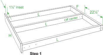
Using deck screws, assemble the base of the staircase by attaching the lower width support (F) to the two outside depth supports (L). Secure the off-center depth support 22½" from the left edge. Using drywall screws, attach the front riser (H) but inset each end by 1½" as shown
